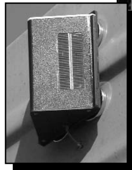
Old cars get new abilities. A mobile wireless system manufactured by Denver, CO-based Lat-Lon LLC is enabling Union Pacific to monitor conditions even on its older reefer rail cars.
